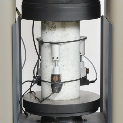
Specimen fitted with 55-C0222/F compressometers
