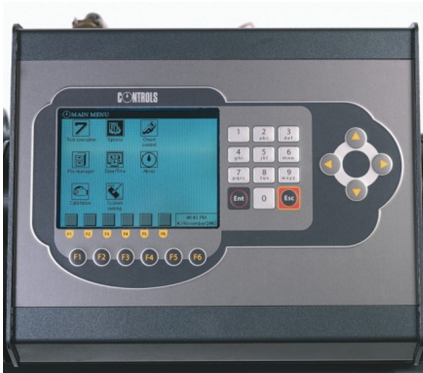
Detail of MCC display used basically for calibration purpose
